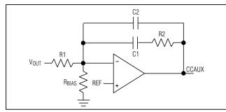
Figure 6. Type 2 Compensation Circuit
