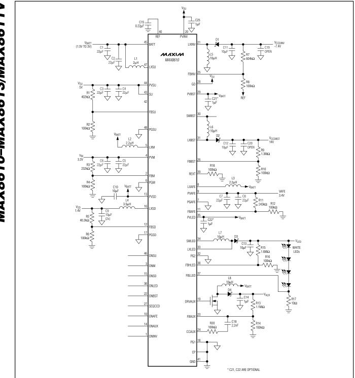
Figure 1. MAX8610 (2 AA Input) Typical Application Circuit. The MAIN and AFE outputs operate as step-up converters.
