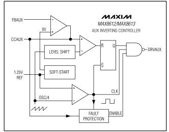
Figure 5. AUX Inverter-Controller Block Diagram
