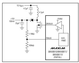
Figure 8. Typical Application for the AUX Boost Controller on the MAX8610/MAX8611/MAX8611V
