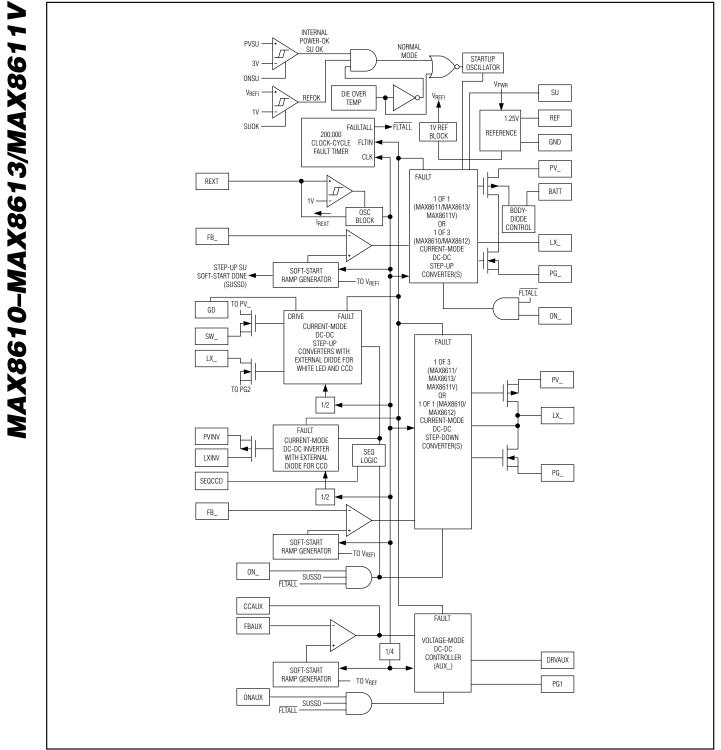
Figure 3. MAX8611 Functional Diagram
