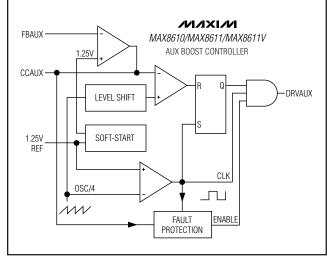
Figure 4. AUX Boost-Controller Block Diagram
