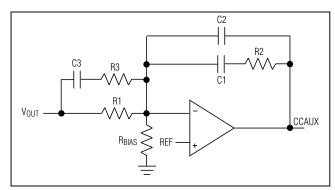
Figure 7. Type 3 Error-Amplifier Circuit
