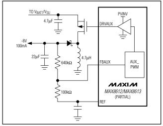
Figure 9. Typical Application for the AUX Inverting Controller on the MAX8612/MAX8613
